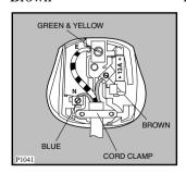
The wire coloured green and yellow must be connected to the terminal marked with the letter  $\ll E \gg$  or by the earth symbol  $\frac{1}{2}$  or coloured green and yellow.
